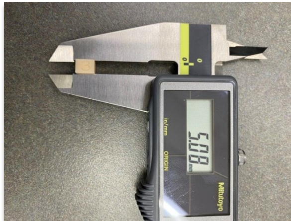
Figure 15. Calipers measuring calibration Cube 3.
